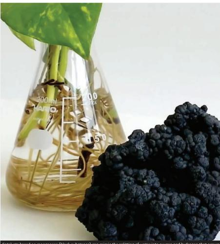
Catalysts based on manganese (black substance) can mimic the splitting of water into oxygen and hydrogen that occurs in plants inside the photosystem II protein cluster responsible for photosynthesis.
